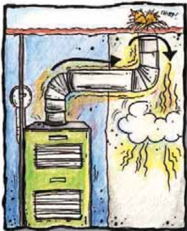
Blocked furnace vent
